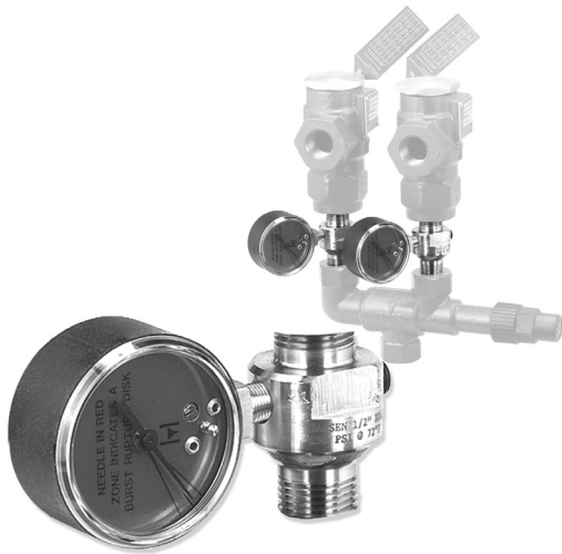
Rupture Disc Assembly with Pressure Gauge Installed Between 3-Way Valve and Pressure-Relief Valve
