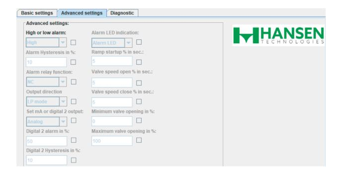
**High or Low Alarm:** High alarm triggers when the level gets above the Alarm setting % and Low alarm triggers when level gets below the setting. The Alarm setting % is found in the Basic Settings.
