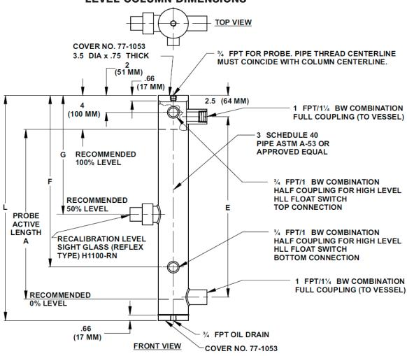
COMPLETE LEVEL COLUMN UP TO 120 (3050 MM) OR PARTS ARE AVAILABLE FROM HANSEN TECHNOLOGIES. PLUGS ARE SUPPLIED FOR THE OIL DRAIN AND FLOAT SWITCH CONNECTIONS.
