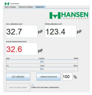
**Zero calibration in pF:** Displays the current 0% reference value.
