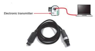
7. Open the Hansen tool and press Start scanning to initiate connection to the sensor. 3 LEDs will display around the M12 connector. Green, red and yellow LEDs will flash when the communication is active.
