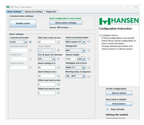
Filter Filter function: time constant in sec.: Filter time averages a period the output over (in seconds) and reduces fluctuations that can lead control. Recommended leave at default value of "20" seconds.
