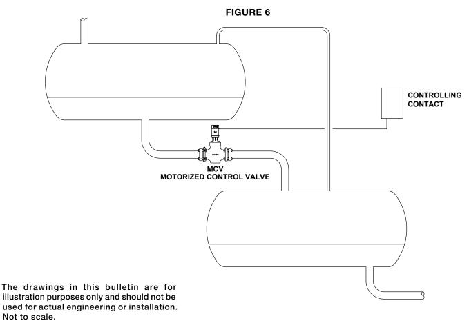
Applications shown use Hansen supplied controllers, however, the Hansen MCV valve series can be integrated into most customer control systems.
