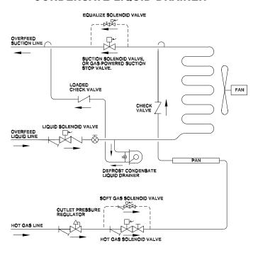
\*For suction closure at temperatures below 0°F (-18°C) alternate low pressure drop valves are preferably used such as Hansen Gas-Powered Suction Stop Valve Type HCK2.
