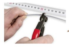
Define the required length of sensor from column. Shorten the wire with wire cutter.
