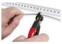
Define the required length of sensor from column. Shorten the wire with wire cutter.
